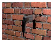
Mark the entry points as specified by the engineer and drill to the correct length using either a core drill or an SDS Max hammer drill.
