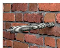
Screw the blanking plug into the end of the first HDS anchor, then insert into the hole. Additional component lengths are then added by simply screwing them together.
