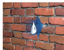
Ensure all debris is removed from the holes using a suitable air pump, then spray with clean water to maximise grout adhesion, and facilitate a gradual and even cure.
