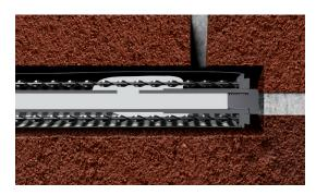
The HDS Sock Anchor system is back-filled, expanding the reinforced mesh sock to completely fill any voids, providing a permanent cementitious fixing to the surrounding masonry.
