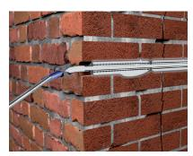
9. When the sock has been fully inflated, milk grout gently runs from the anchor indicating that it's full.
