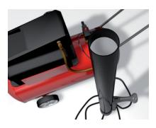
6. Pour the mix into a pneumatic grout gun connected to a compressor set to a maximum of 3 bar pressure.
