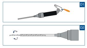
d) Mix the grout are per the manufacturer's instructions and trowel into the injection gun. Pump the grout to the end of the nozzle, then screw the 12mm helical bar into the grout filled nozzle until flush with the end of the nozzle.
