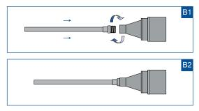
b) Cut the nozzle to the required length (If not previously cut to length) and screw into the threaded top of the three applicator guns. Cox Manuel Gun, Cox pneumatic gun and a cordless Albion gun.
