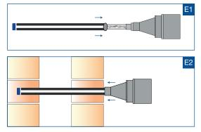
e) Place the sock over the nozzle and pull down the length of the nozzle, then push the sock covered nozzle into the predrilled 22mm hole.
