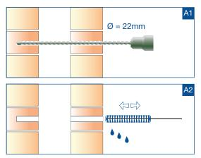
a) Drill a 22mm hole in the substrate to the required depth. Then clean with water and a SureBrush.
