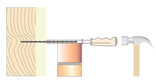
1. Position the tie into the hand held fixing tool as shown above. Drive directly into timber stud through insulation.
