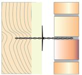
2. Place insulation support over tie, and embed the outer end into the outer leaf mortar.
